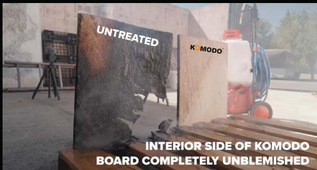
The backside of the Komodo treated OSB board remains completely intact while untreated board has been destroyed.
