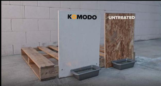
OSB Boards untreated and treated with FireBlock365 prior to burn test at 900 °F.
