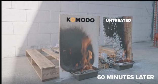
After 60 minutes of continuous burning, Komodo treated board remains structurally unchanged while untreated OSB board has turned to ash.
